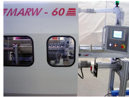
exit conveyor and operator panel
