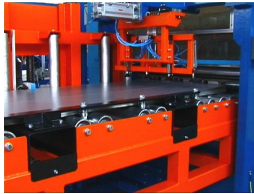
sheet feeder with double sheet detector
